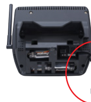
WeatherLinkIP data logger installed in a Vantage Vue console.
